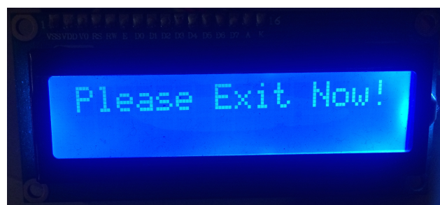
Indicates to the user to leave the building before the system is set to armed.
